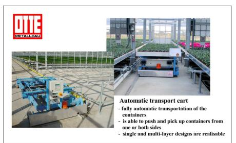
The rail-guided transport cart transports the containers automatically in the cultivation area or in the work area. Each transport cart is designed according to requirements of the customer. Furthermore the automatic transport cart is able to push and pick up containers from one or both sides. Single and multi-layer designs with integrated collection and/or pushing equipment are also realisable.
