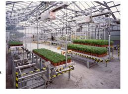
The battery-operated monorail system is excellent qualified for the transport of plants from the work area in the cultivation area and back again. The rail-guided monorail system could be arranged with slide switches or turnstile switches. This system is available with manual or automatic control.
